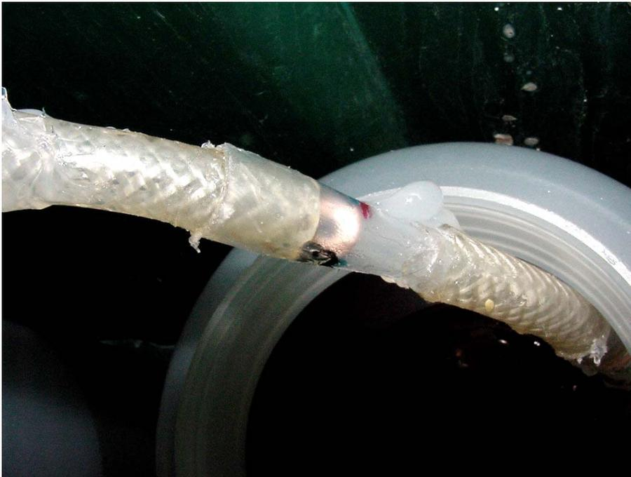
Figure 2. Close up of sample holder. Copper sample is visible through clear plastic tubing.
